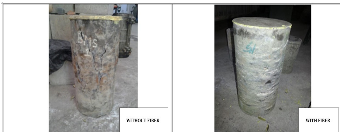
Fig. 9. Crack Pattern after Compressive Strength Test
