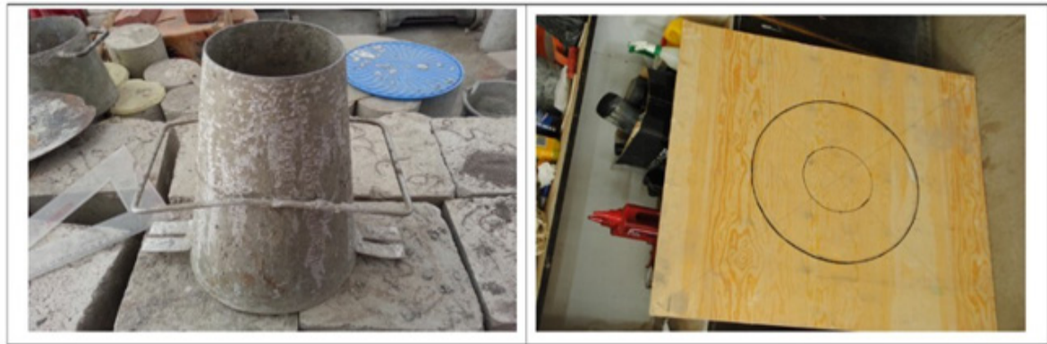
Fig. 2. Abarms Cone for Slump Flow Test
