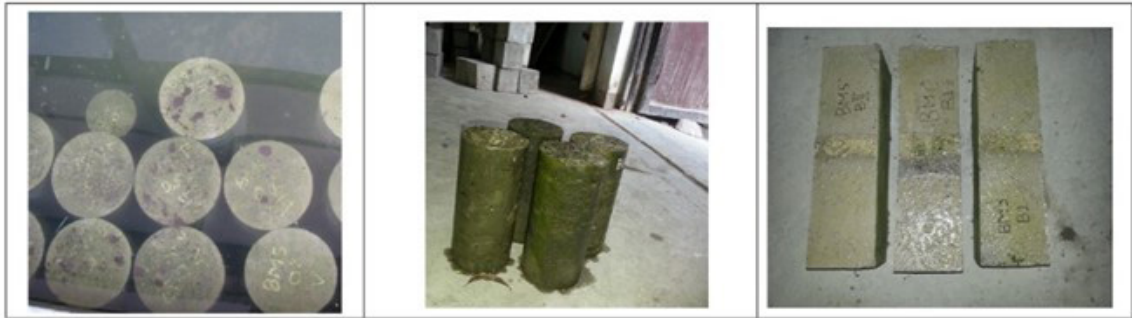
Fig. 3. Curing Concrete Specimen
