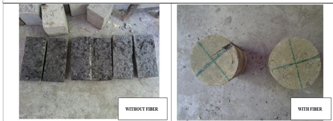
Fig. 10. Crack Pattern after Splitting Tensile Test
